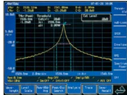
Measurement of optical band pass filter
